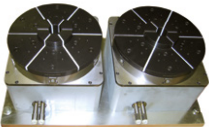
Example of a double unit MX \varnothing = 400 mm with customer specific sealed segment jaws, for the machining of sensitive rings
