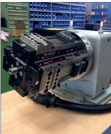
Lehmann dividing head with Trigo tower clamping system
