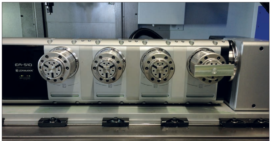
4-way set-up for dividing head
