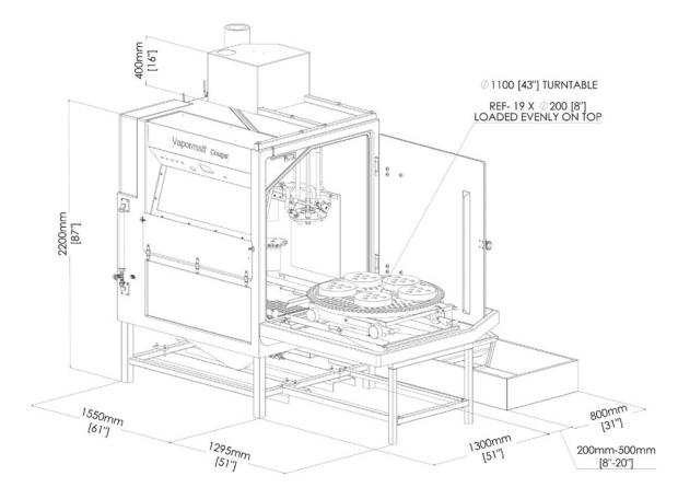
The Vapormatt Cougar Radial automatic machine provides an entry level solution for production facilities requiring automated wet blasting facilities.
